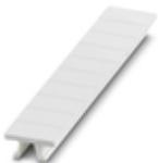
Zack marker strip, Strip, white, unlabeled, can be labeled with: PLOTMARK, CMS-P1-PLOTTER, mounting type: snap into tall marker groove, for terminal block width: 5.2 mm, lettering field size: 5.1 x 10.5 mm, Number of individual labels: 10
