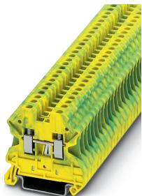
Ground modular terminal block, connection method: Screw connection, number of connections: 2, cross section: 0.14 mm<sup>2</sup> - 4 mm<sup>2</sup>, AWG: 26 - 12, width: 5.2 mm, height: 46.9 mm, color: green-yellow, mounting type: NS 35/7,5, NS 35/15
